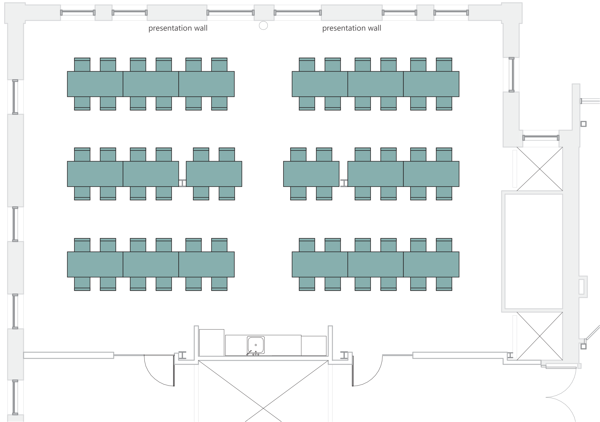
Program Room 301 - Plan Layout A Tables & Chairs / Face-to-Face Seating / Horizontal Orientation: 72 Seats
